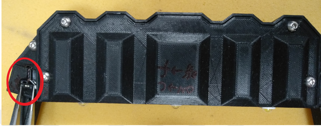
Figure 3.4: The stimulator part of the 3D printed headset: The button to select the stimulation modality (f-VEP or c-VEP) is encircled
