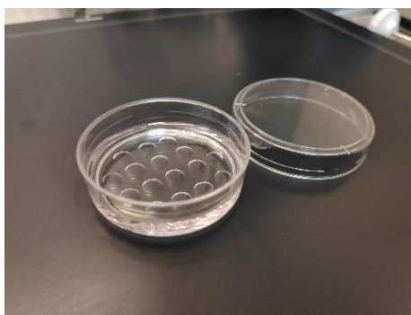
Figure 21. Embryo culture plate. 10 \mu\text{l} embryo culture drops were placed on the 35 mm culture plate surface and mineral oil was overlaid on the culture drops to inhibit evaporation and contamination.
