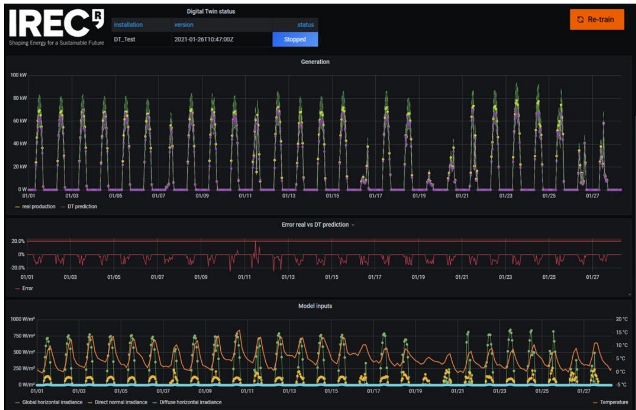
Figure 4. 16 Dashboard in grafana with model input data with grid part
