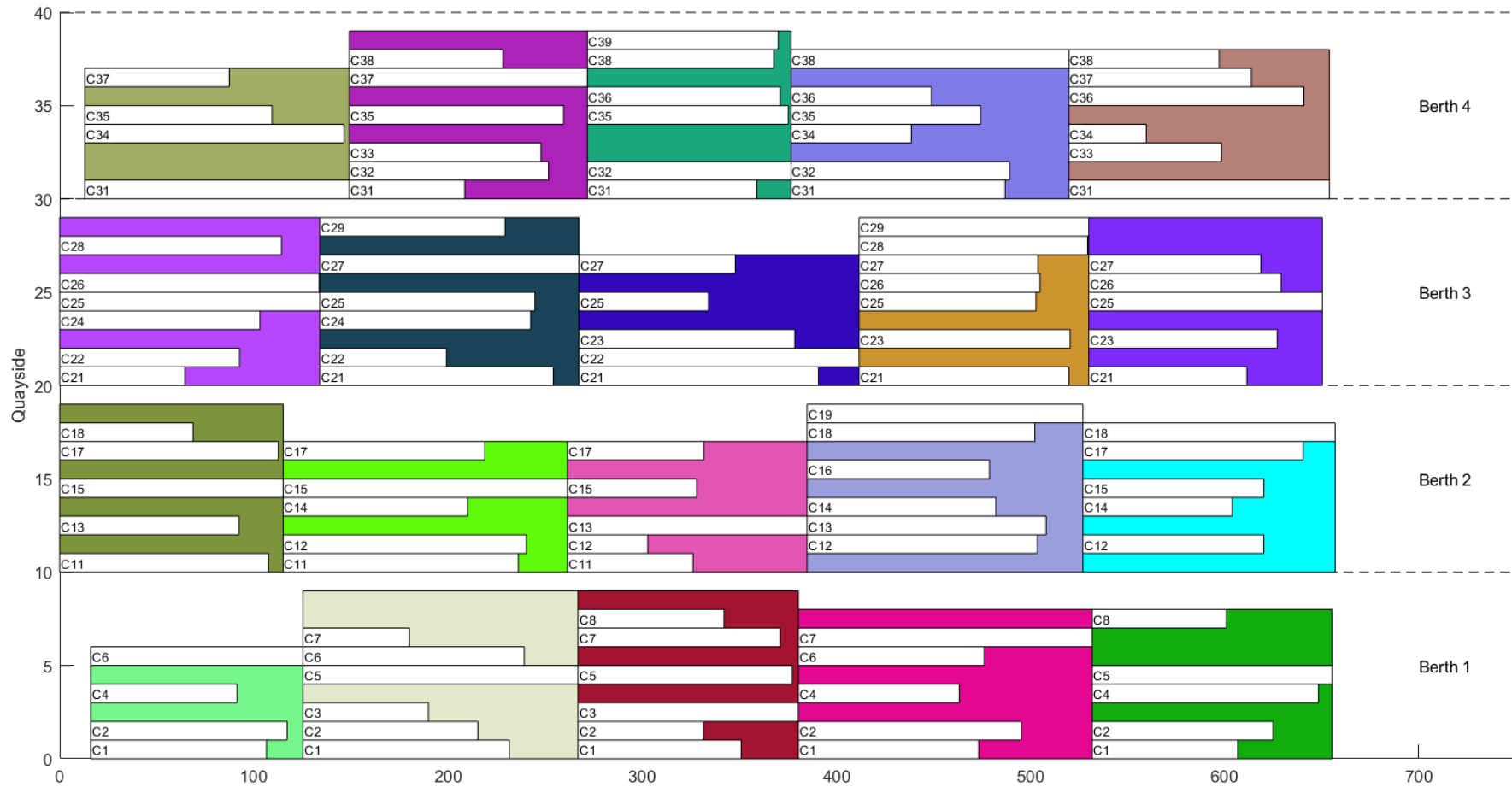
Figure 4.4 Berth space-time diagram for the solution of the sample problem 1 when it is not crane-constrained
