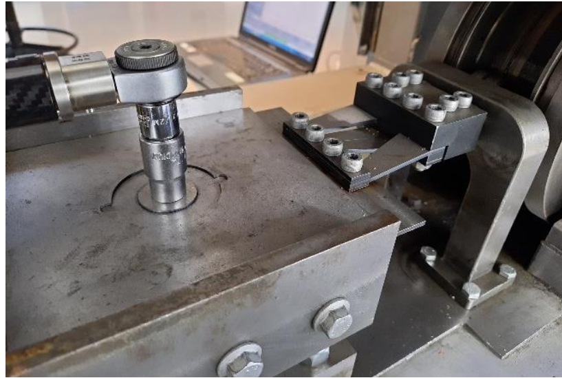
Figure 3.4 Bolt installation in Junker vibration test device with Atlas Copco ST Wrench
