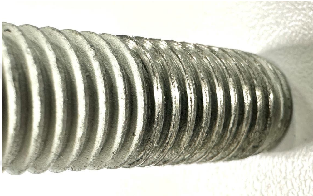
Figure 4.9 Worn threads due to multiple re use
