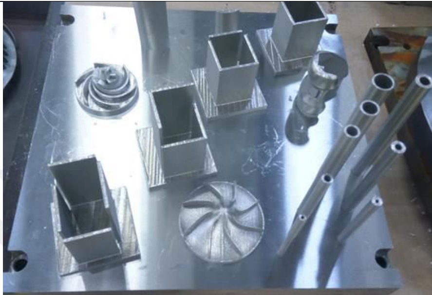
Figure 5-14- Parts manufactured via EOS M290 additive manufacturing machine
