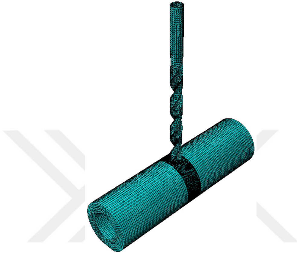
Figure 2.7: Finite Element Model of the Bone-Dental Drill Assembly
