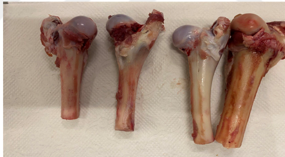
Figure 3.2: Cleaning of femur specimens to remove soft tissues and maintain hydration.
