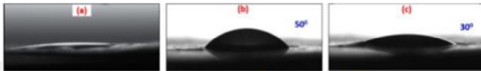
Figure 2.17. Images of water droplets on collagen scaffolds (a) uncrosslinked, (b,c) crosslinked captured at different time after droplet deposition (Kitsara et al., 2015)
