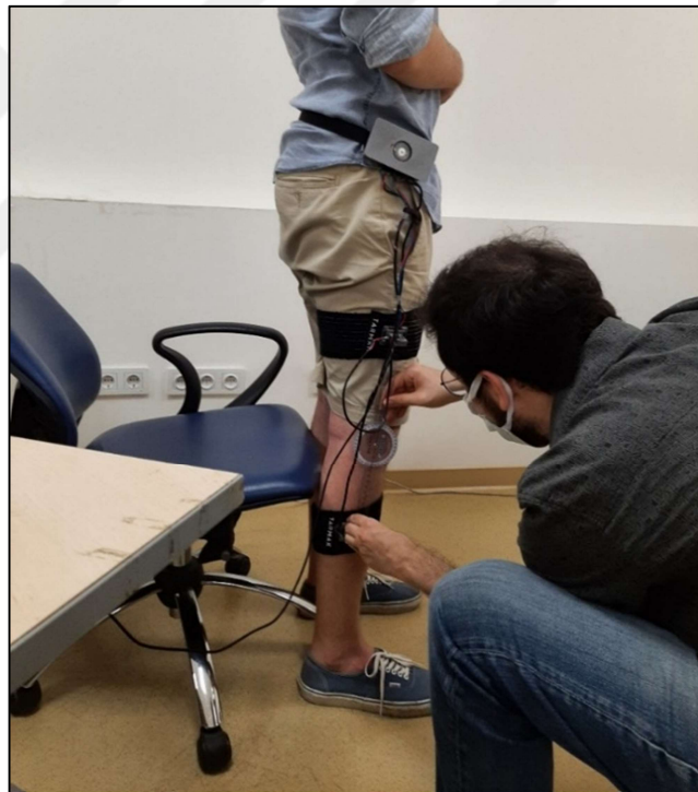
Figure 2.10. Knee range of motion and sensor placement control
