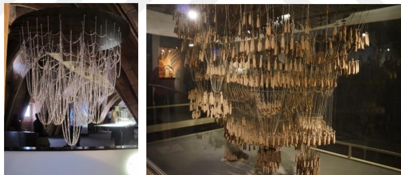
Figure 2.4. (1,2) Hanging chain models of Gaudi for Sagrada Familia ( http://dataphys.org/list/gaudis-hanging-chain-models/ )
