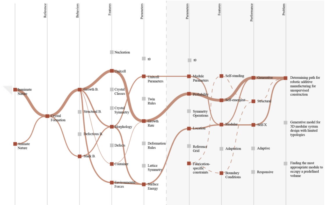
Figure 4.11. Mapping between crystal formation and path detection problem for robotic additive manufacturing.
