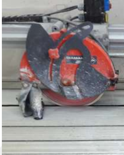
Figure 2.7 Wet cutting saw
