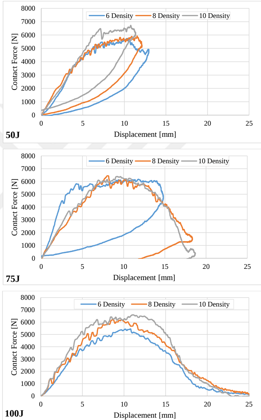
Figure 3.13 Contact force-displacement graphics according to the density for different impact energies
