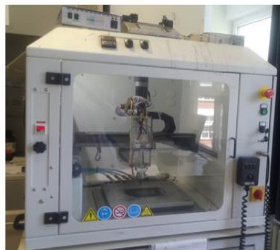
Figure 0.38. Fuel cell test system and the Sonotek ExactaCoat spray device
