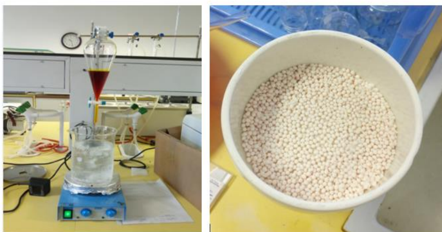
Figure 0.28. sPEEK precipitation in ice cold water and the washed samples
