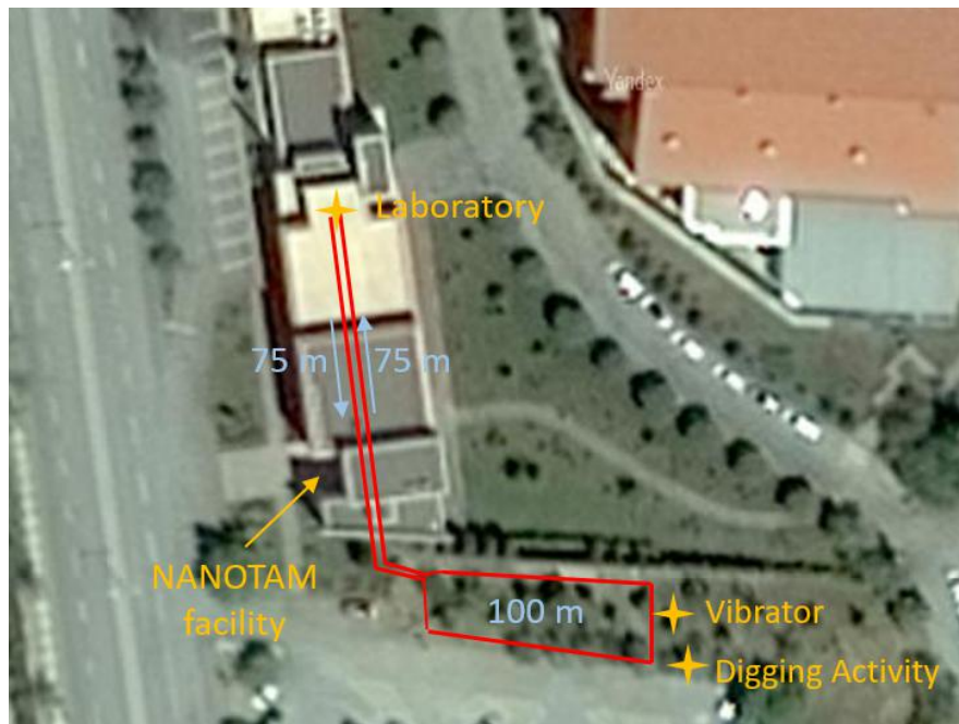
Figure 5.1: Test field with buried fiber cables around NANOTAM facility.
