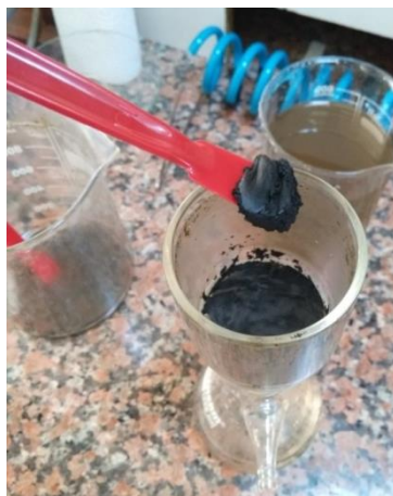
Figure 3.5 The remaining solid GO in the Gooch crucible after completion of the vacuum filtration (Personal archive, 2018)
