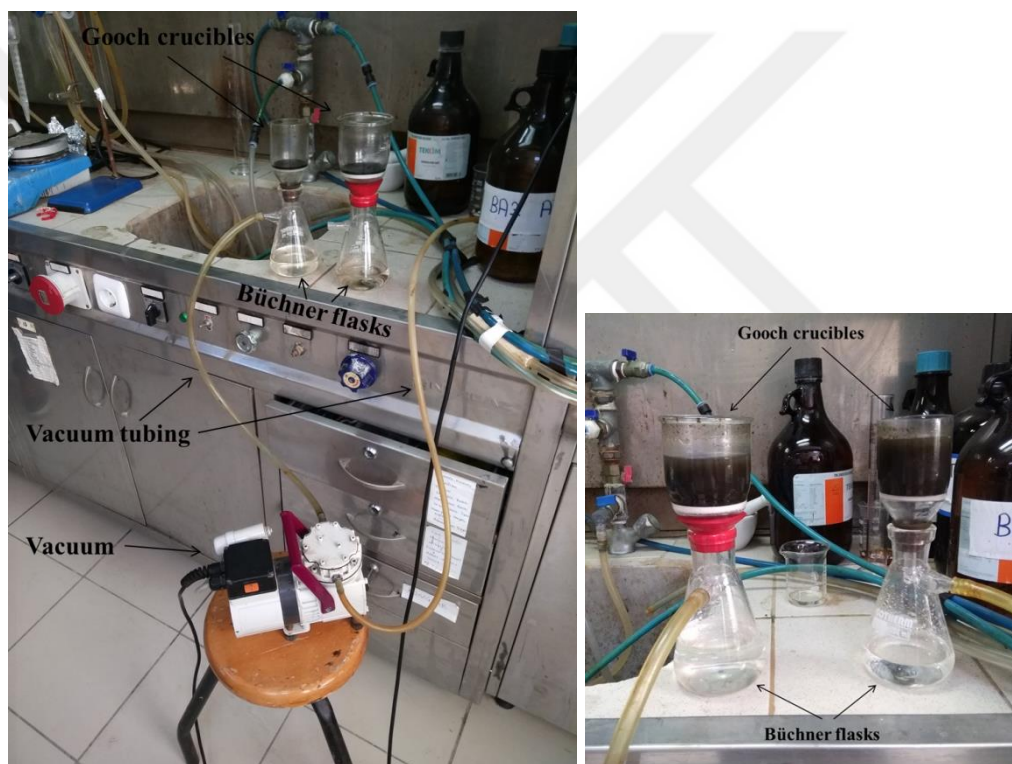
Figure 3.4 The vacuum filtration setup used (Personal archive, 2018)
