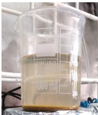
Figure 3.3 The obtained precipitate after standing overnight (Personal archive, 2018)
