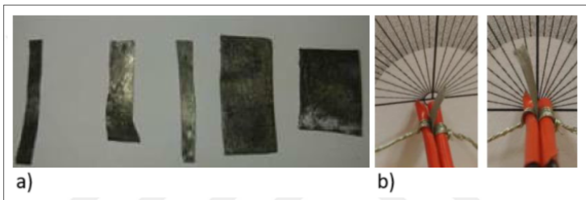
Figure 2.15 a) Produced ionic electro-active polymers. b) Right and left bending motions of the IEAP when voltage is applied.
