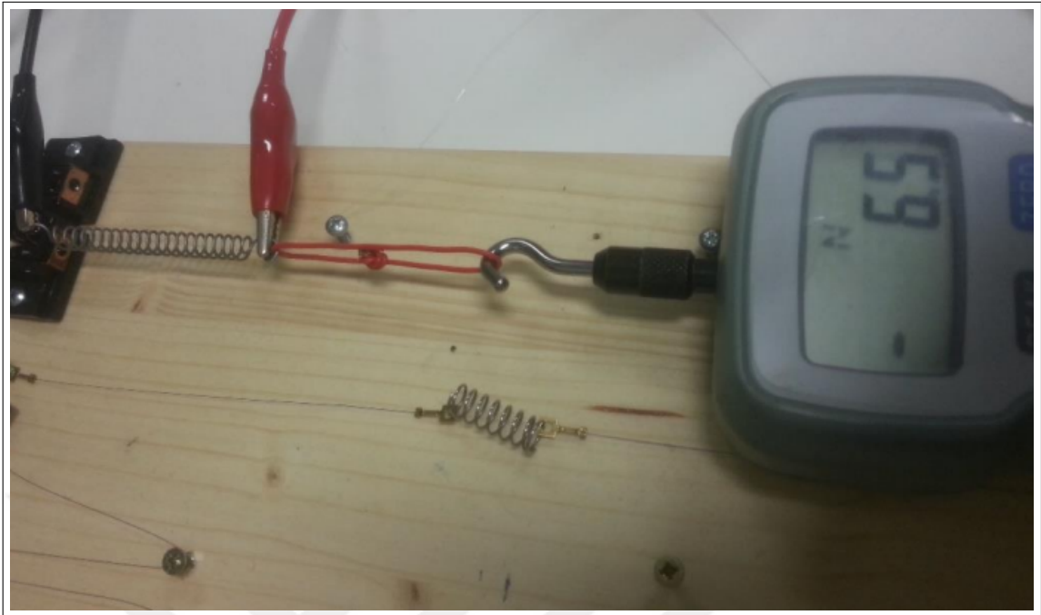
Figure 3.14 Detailed view of spring load testing mechanism. Detailed view of a palm-sized digital force gauge used in early-stage spring load measurements. The SMA spring is attached between fixed and moving ends, and the force is recorded as the spring contracts upon electrical activation. This compact device enabled practical measurements before transitioning to an integrated load cell system.
