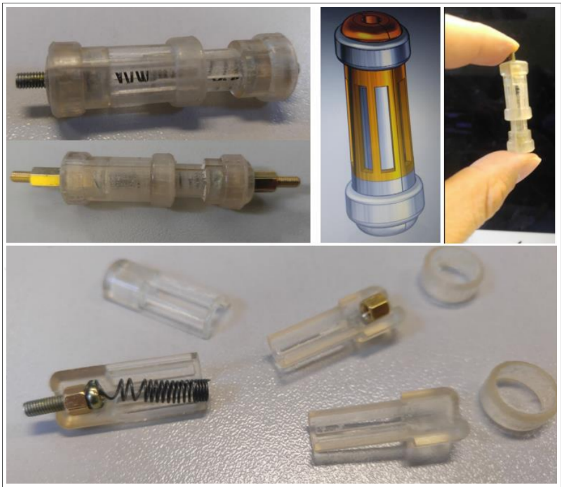
Figure 3.6 Standalone SMA actuator prototype designs fabricated for controlled modeling experiments.
