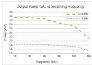
Fig 4: Output Power (SiC) vs Switching Frequency at AC Input
