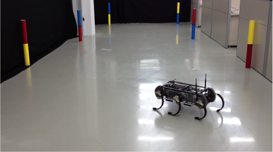
Figure 3.9: A snapshot from the experimental setup in its initial state. Six colored landmarks are scattered throughout the environment, observable through a camera mounted on the RHex robot.
