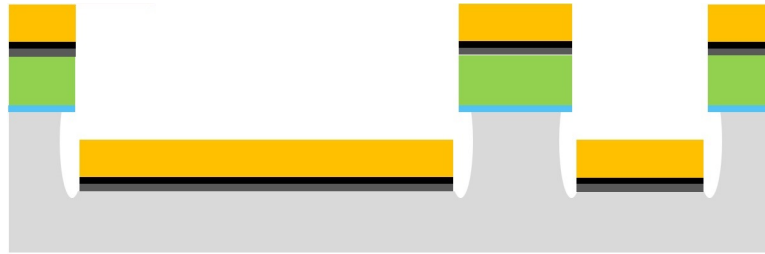
Figure 2.56: Metallization (Ti-Pt-Au) as the bottom electrode.
