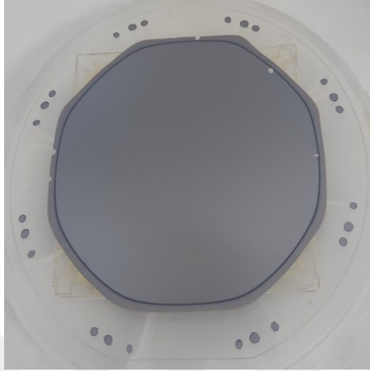
Figure 2.13: Pyrex-SOI wafer pair after complete the removal of BOX layer (with Si-device layer on top).
