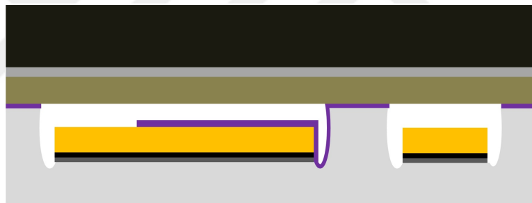
Figure 2.66: Anodic Wafer Bonding of Pyrex and Silicon-on-Insulator (SOI) wafers.
