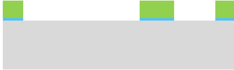
Figure 2.53: Argon Reactive Ion Etching (RIE) for etching chrome hard mask.
