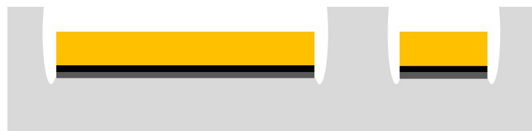
Figure 2.58: Chrome wet-etching using chrome etchant.
