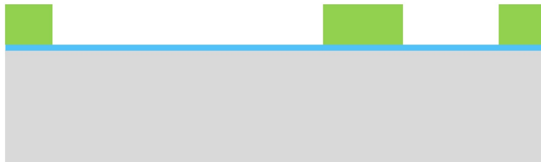
Figure 2.52: Photolithography with Mask 1 for cavity formation on Pyrex wafer.
