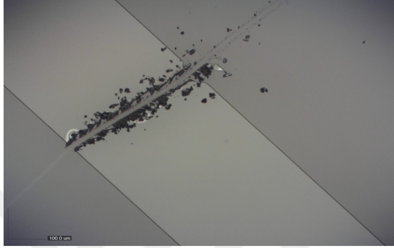
Figure 2.24: Photoresist feature on the Silicon test wafer underwent the Scratch Test after photoresist development.
