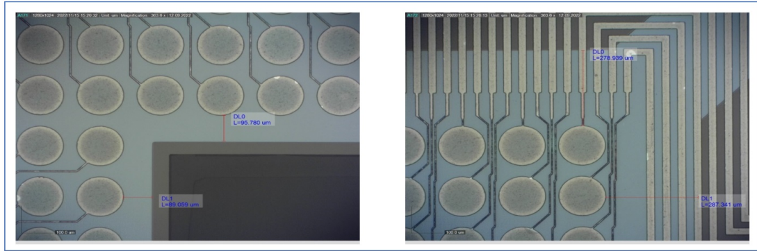
Figure 2.28: Optical microscope images displaying alignment accuracy measurements of the photoresist mask (Mask 4) on corner CMUT chips of the Pyrex-SOI wafer pair. Note: These optical images are taken from the back side of the Pyrex wafer, after Si device layer was also etched. Although not shown here, similar alignment accuracy inspection has been done on the corner chips from the front side of the Pyrex wafers before all the wet etching and Bosch process Si etching steps were performed, because all these etch processes are irreversible patterning processes.
