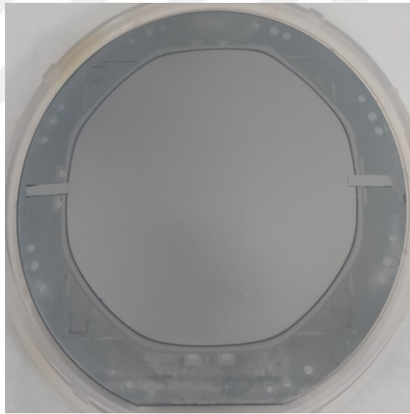
Figure 2.16: Pyrex-SOI wafer pair after blanket deposition of Cr-Au-Cr layers.
