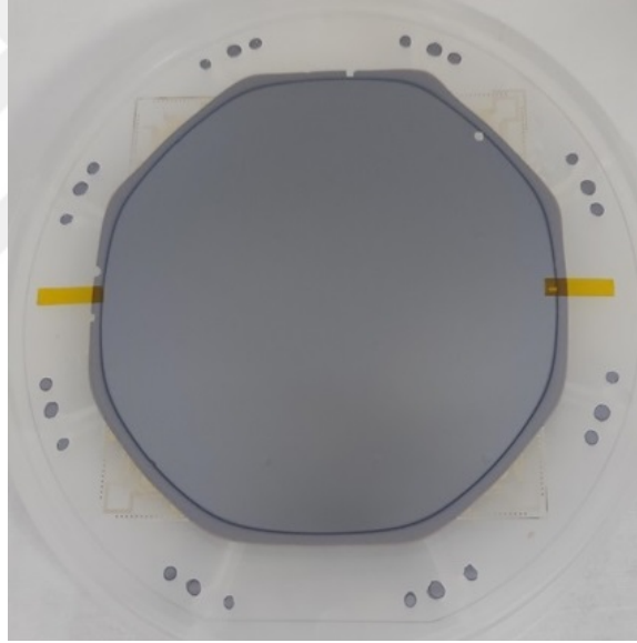
Figure 2.15: Pyrex-SOI wafer pair after masking its alignment marks with the Kapton tape.
