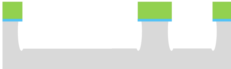
Figure 2.55: Buffered Oxide Etch (BOE) wet-etching process for Pyrex. Note that the undercut below the photoresis is increased, and depth of the gap is also increased.
