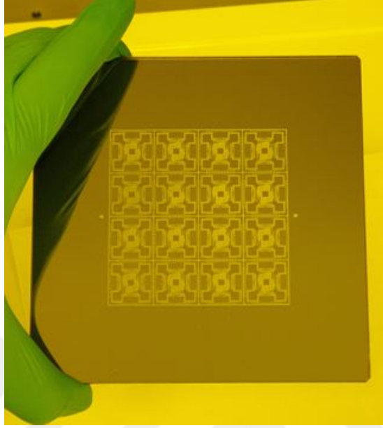
Figure 2.16: A photograph of the used cavity formation mask during microfabrication process.
