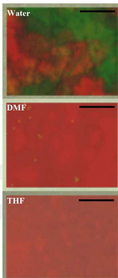
Figure 2.5. Raman mapping of synthesized calcium phosphate phases (scale bar=20 \mu\text{m} ), HA (red), \beta -CPF (green)
