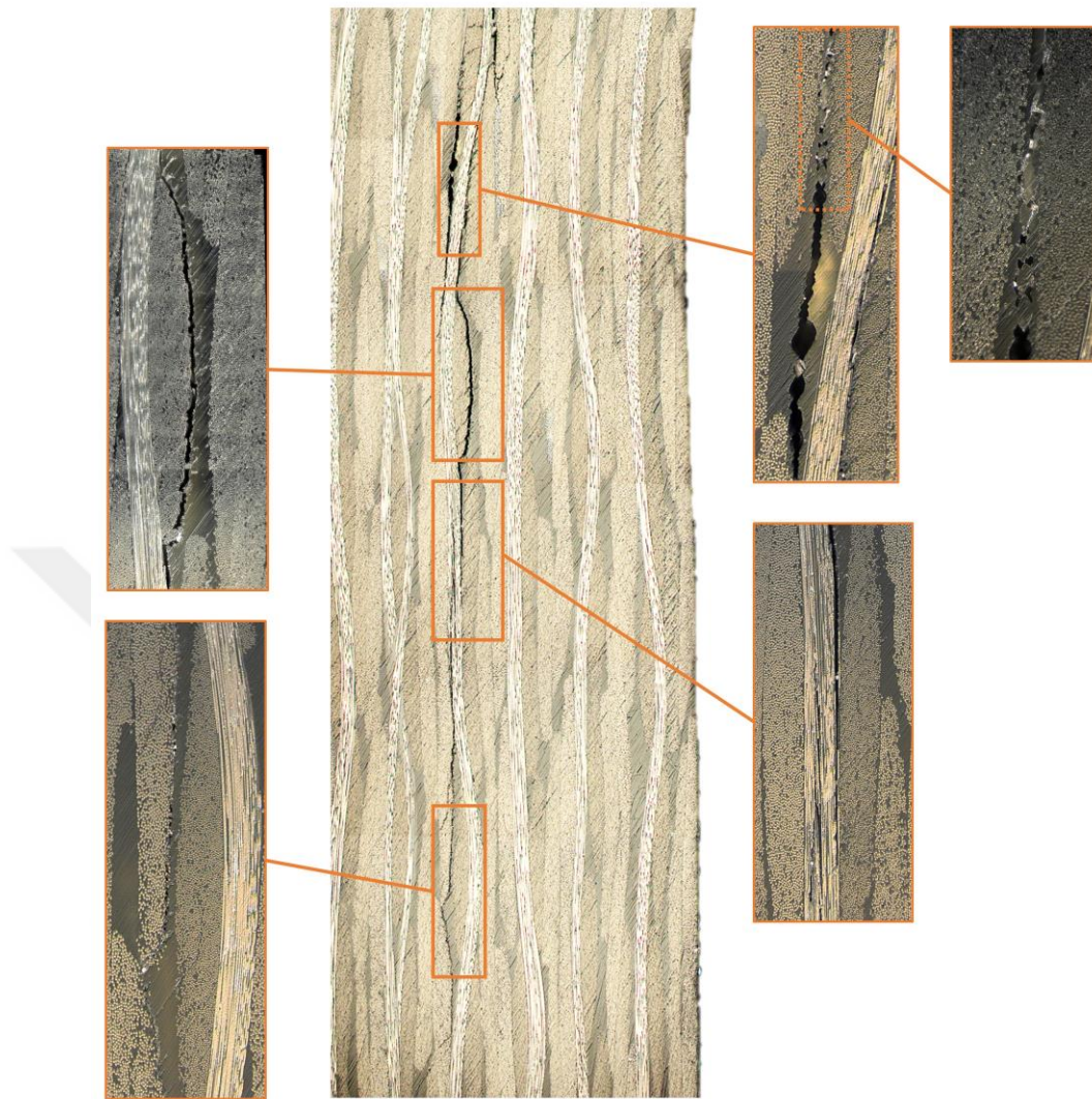
Figure 5.16. Post-mortem micrograph taken from the vertical arm of Fabric 3.
