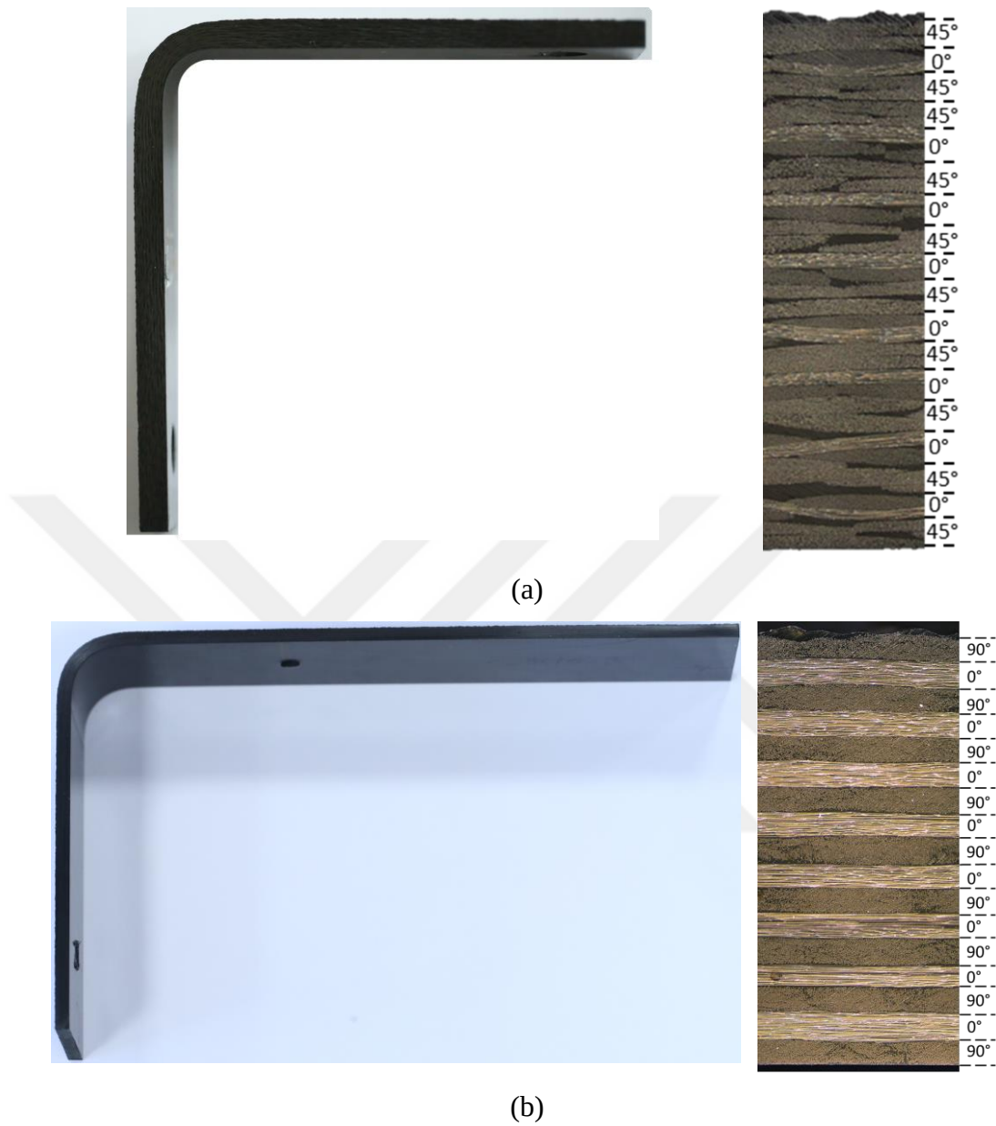
Figure 3.2. Sample specimens and microscopic views of their stacking sequences: (a) Fabric specimen, (b) cross-ply specimen
