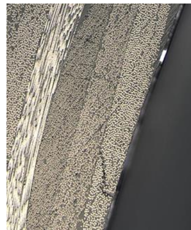
Figure 5.10. Detailed micrographs of the matrix cracks observed in the Fabric 1.
