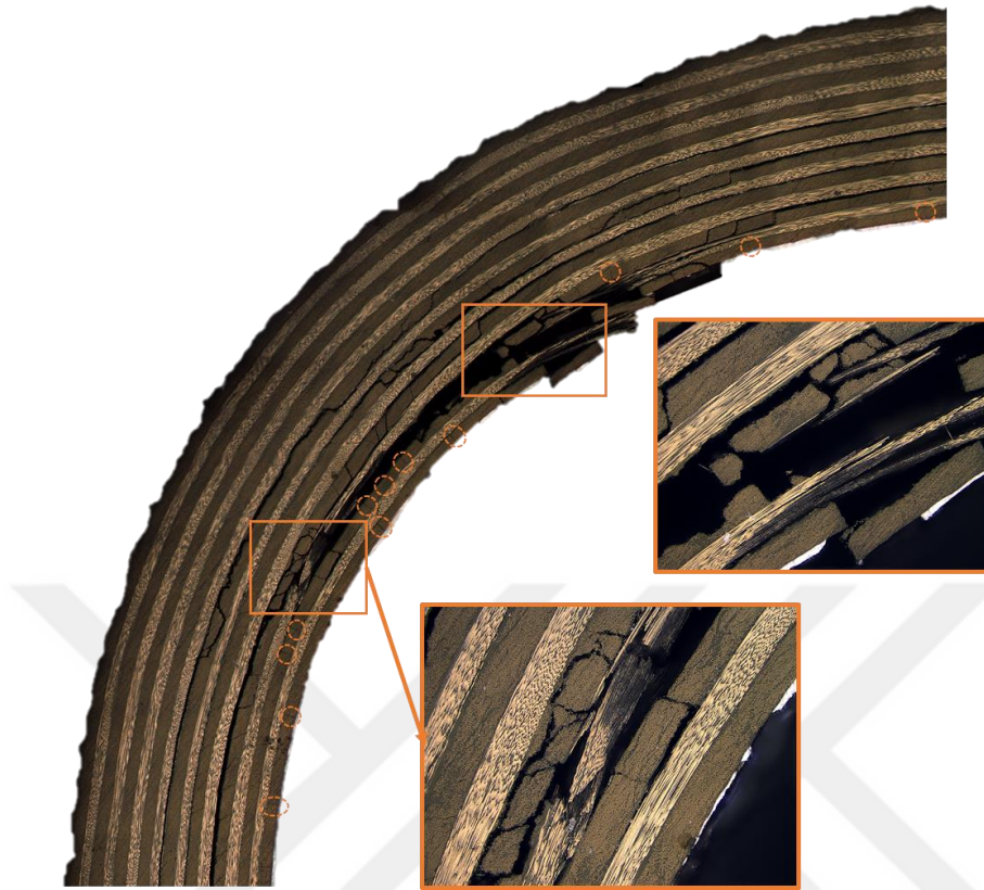
Figure 4.14. Post-mortem micrograph taken from the curved region of specimen 90/0-8
