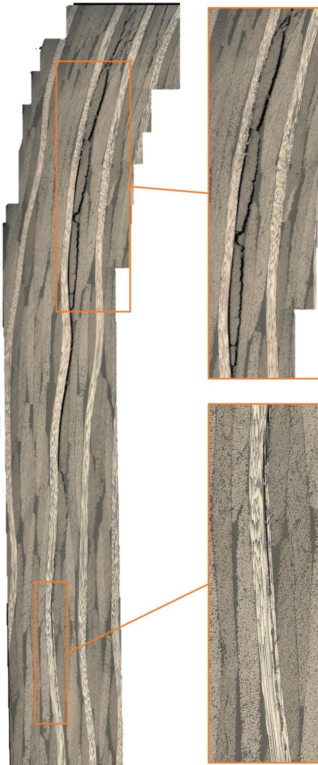
Figure 5.13. Post-mortem micrograph taken from the vertical arm of Fabric 1.
