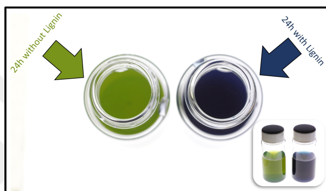
Figure 30. Prussian blue reaction. Visual comparison of the blank sample (without lignin) and lignin contained sample (polyphenol) after 24 hours .
