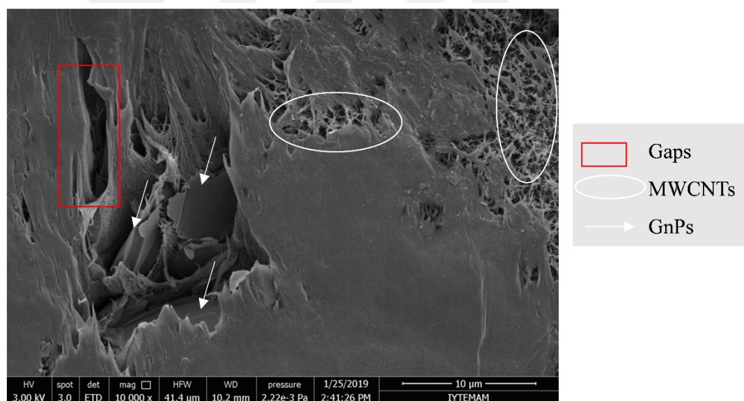
Figure 7.8 SEM image of the HDPE/G3/M12 nanocomposites with 1/4 weight ratio of GnPs/MWCNTs (5wt.%) (10 000 ×)
