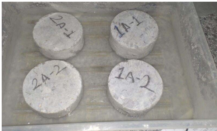
Figure 2.9 Capillary water absorption test specimens
