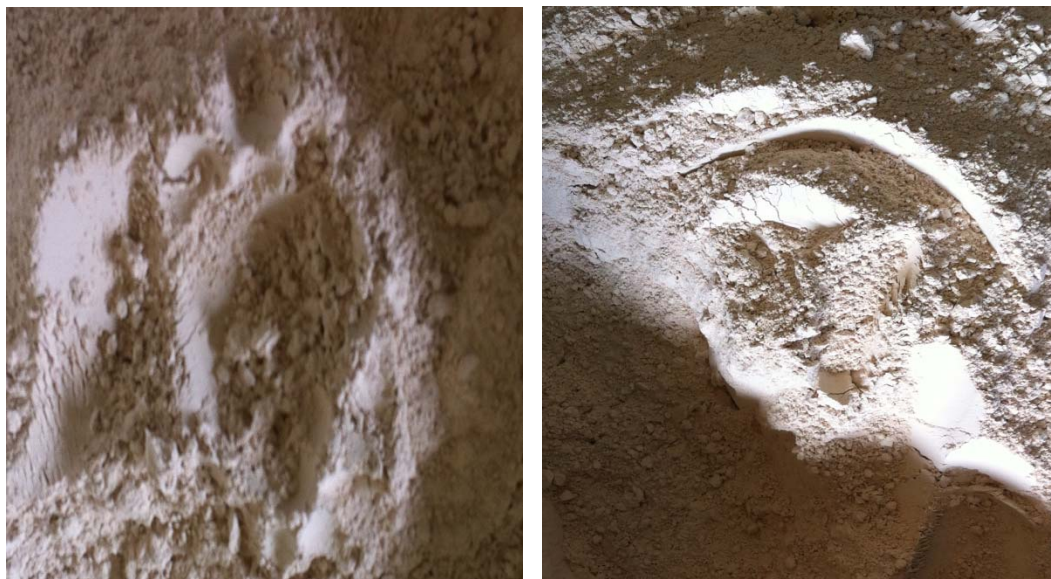
Figure 2.2 Fine aggregate below 63 \mu\text{m}
