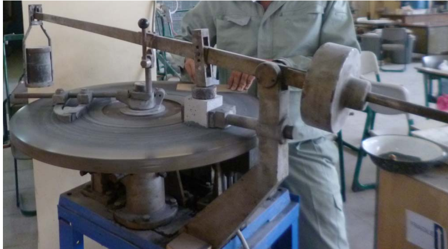
Figure 2.11 Bohme abrasion devices
