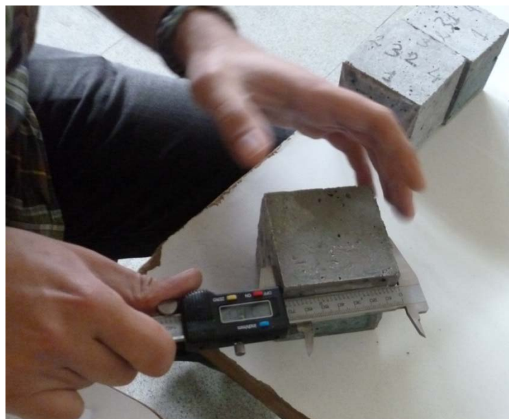
Figure 2.12 Measurement after cycling
