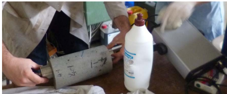
Figure 2.14 Ultrasound test for cylinder specimen
