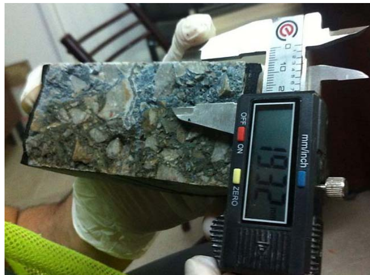
Figure 2.21 Measuring the depth of chloride-ion penetration from a half slice of specimen
