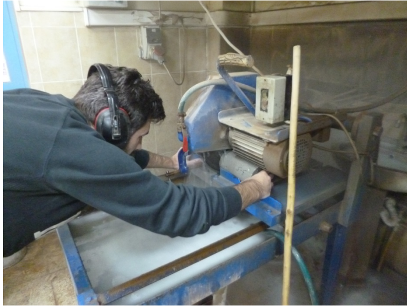
Figure 2.18 Cutting slice from specimen after 28 days curing
