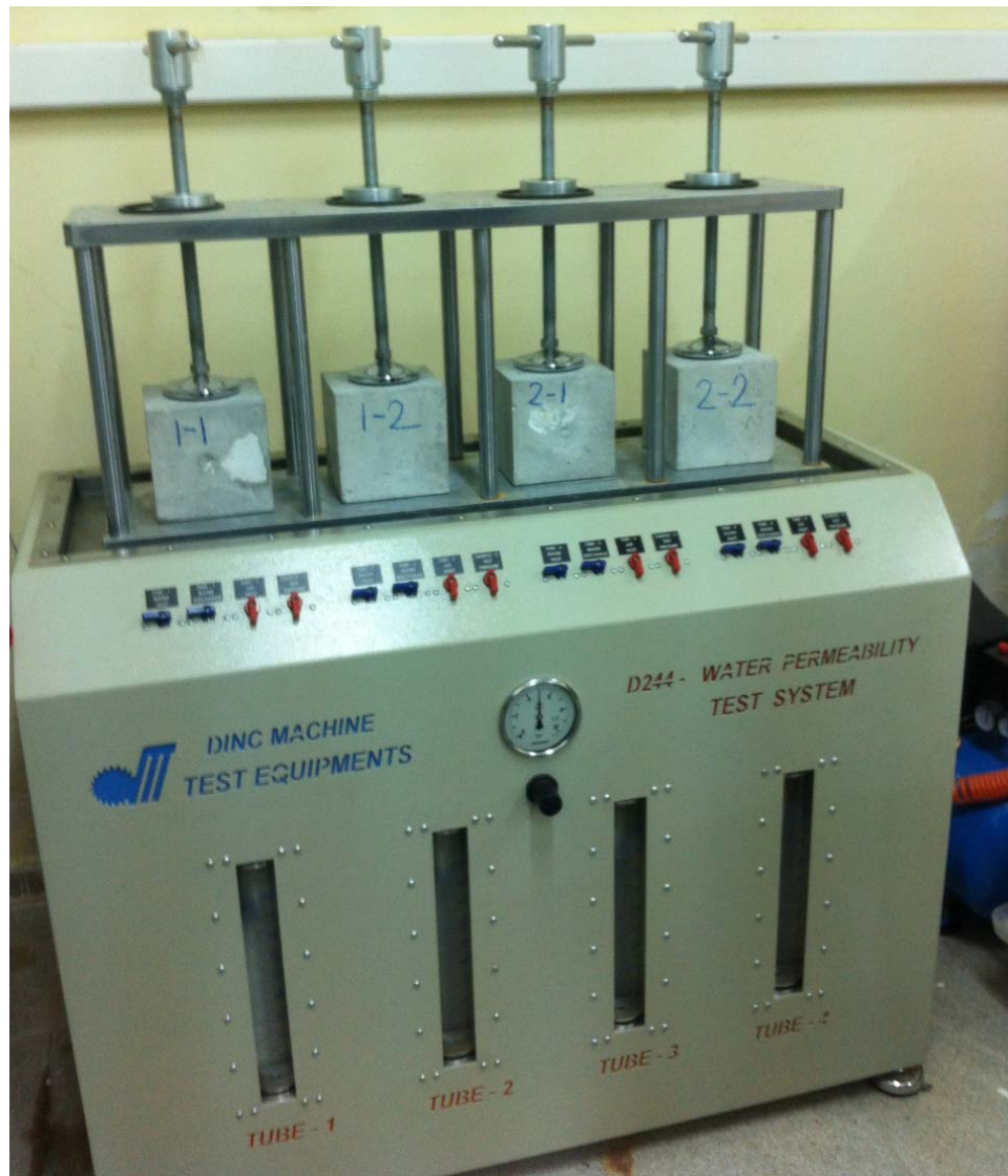
Figure 2.22 Water penetration depth test device
