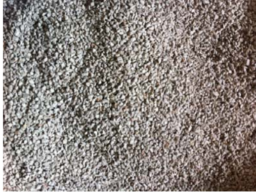
Figure 2.3 Fine aggregate below 250 \mu\text{m}
