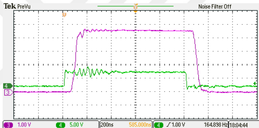
Figure 5.6. 500 V output waveform with 1 \mu s width by a PCB which is waveform 3.
