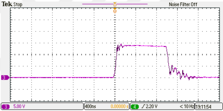
Figure 6.39. Output waveform of the three cascaded Marx generator units supplied by 500 V
