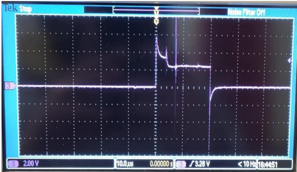
Figure 5.3. Homemade cascaded PCB output result which is controlled by Arduino Uno
