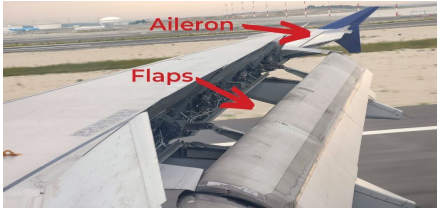
Figure 1.3. Illustrates aileron and flap control panels in an aircraft [2]
