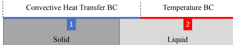
Figure 3.4: Modification for heat transfer BC of condensation
