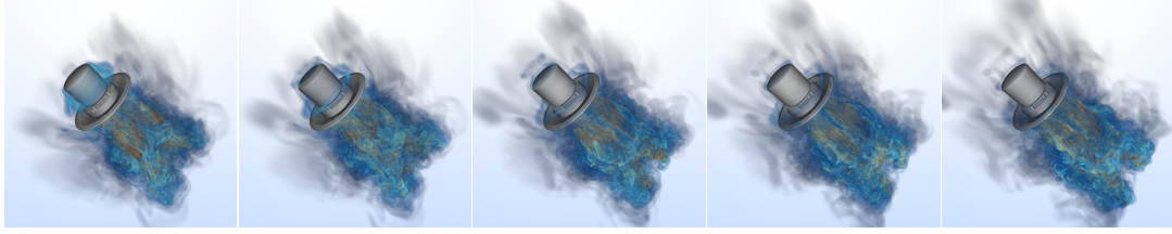
Figure 5.1: Data-parallel rendering of the “Small Mars Lander” computational fluid dynamic data set, which comprises 72 clusters of finite elements. The images are rendered on 18 compute nodes and 72 NVIDIA Quadro RTX5000 GPUs of the Frontera RTX partition at the Texas Advanced Computing Center (TACC). The image resolution is 1024 \times 1024 . The average frame rate of this image sequence is around 15.00 fps.
