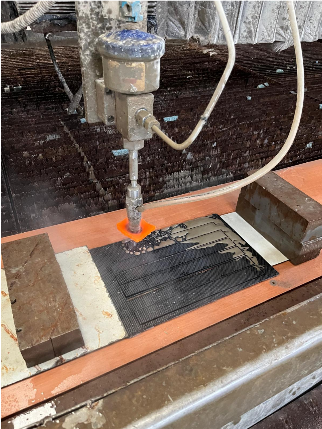
Figure 3.5. Cutting the tensile and vibration test specimens using water jet
