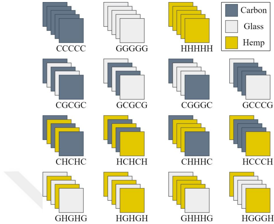
Figure 4.13. Stacking sequences of laminated composite plates.
