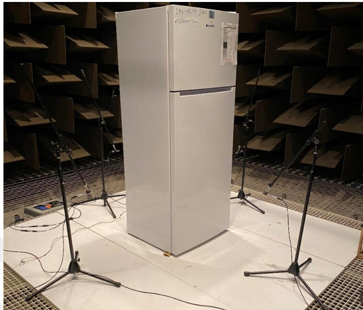
Figure 3.28. Sound pressure level measurement in full anechoic room
