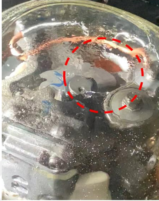
Figure 1.11. Oil splash as the crankshaft rotates in clockwise.
