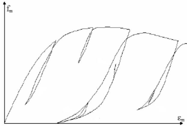
Figure 4.7 Hysteretic Model for Axial Cyclic Behavior (Crisafulli, 1997)
