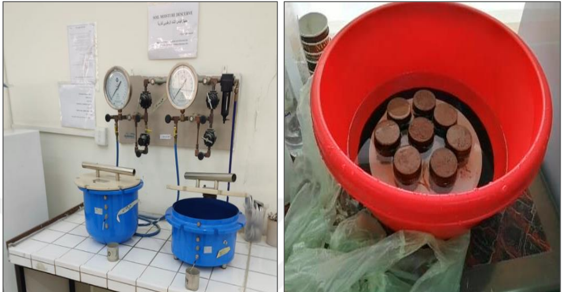
Figure 3.8 Soil field capacity and permanent wilting point analyses (Original 2022)
