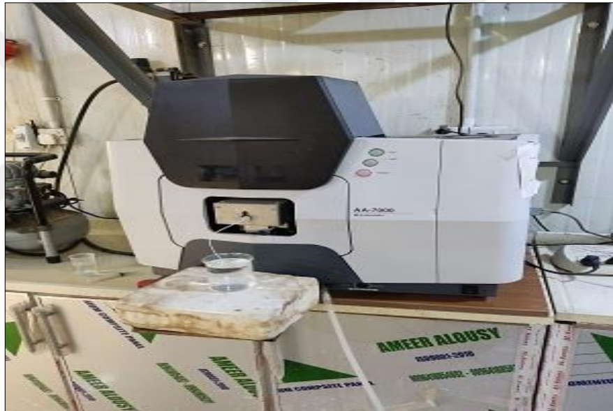
Figure 3.12 Atomic Absorption Spectrophotometry (AAS) used for metal analysis (Original 2022)
