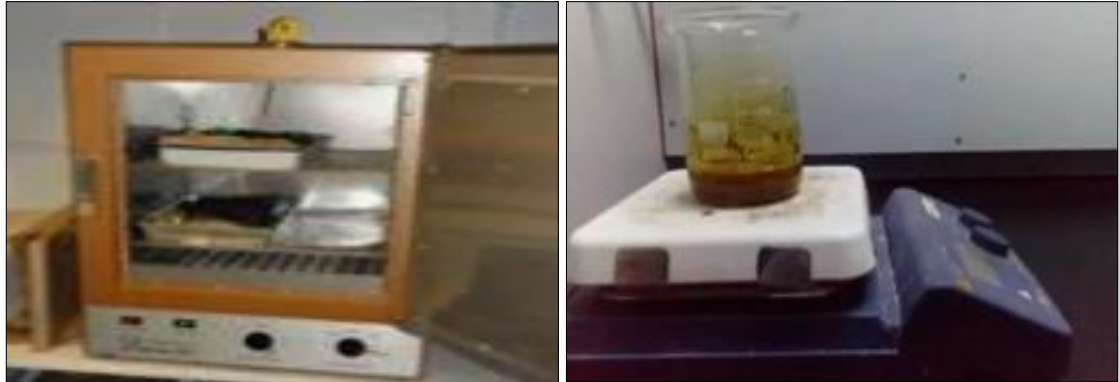
Figure 3.11 Preparation of soil samples for metal analysis (Original 2022)
