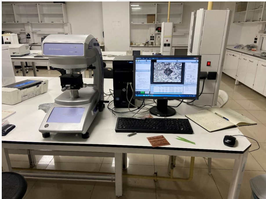
Figure 2.12 The hardness measuring device used in the tests
