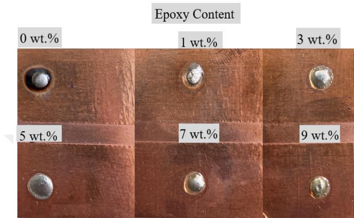
Figure 3.6 Sn-Bi solders with different epoxy content
