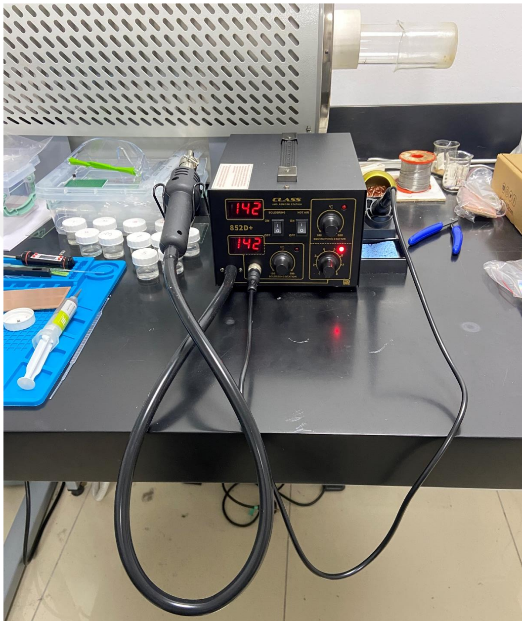
Figure 2.4 Heat-blown soldering iron used
