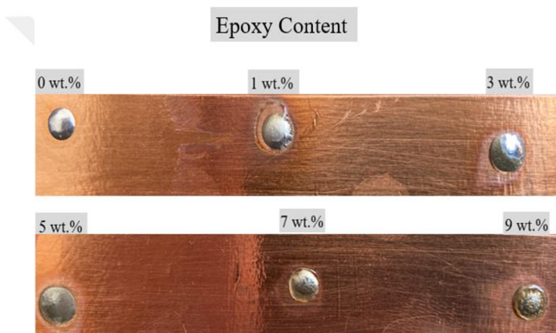
Figure 3.5 Sn-Bi solders with different epoxy content
