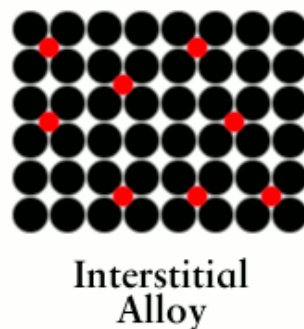
Figure 2.2 Interstitial alloy (as the reds are smaller size agent atoms in between the black base atoms) [10].
