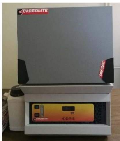
Figure 5.3 The furnace that's used for homogenizing the samples
