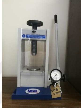
Figure 5.1 The pressing machine that we used to press the powdered elements and make it as pellets.
