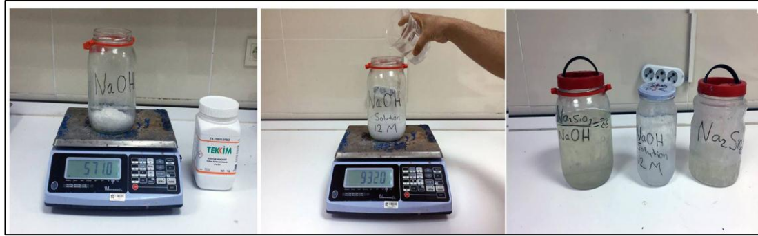
Figure 3.1 Preparing alkaline activator
