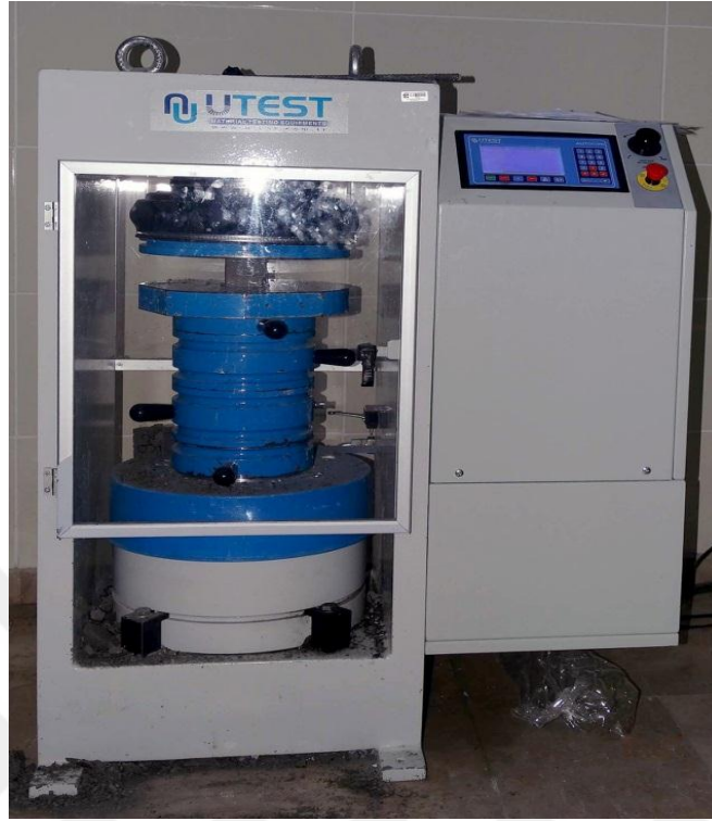
Figure 3.9 Compressive strength test
