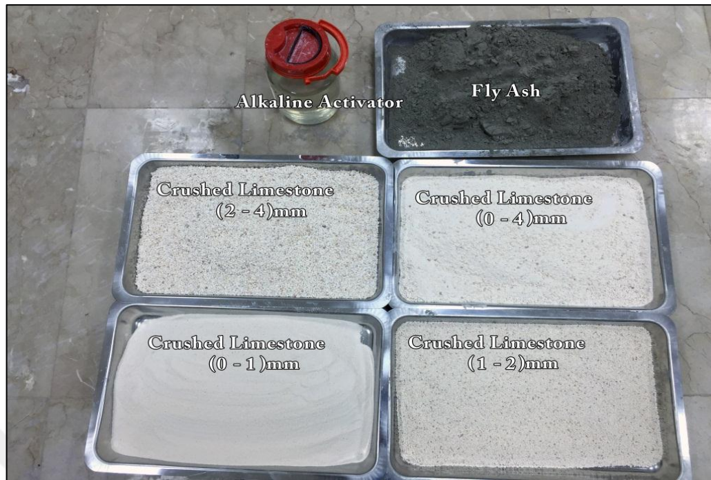
Figure 3.3 Preparing geopolymer mortar constituents
