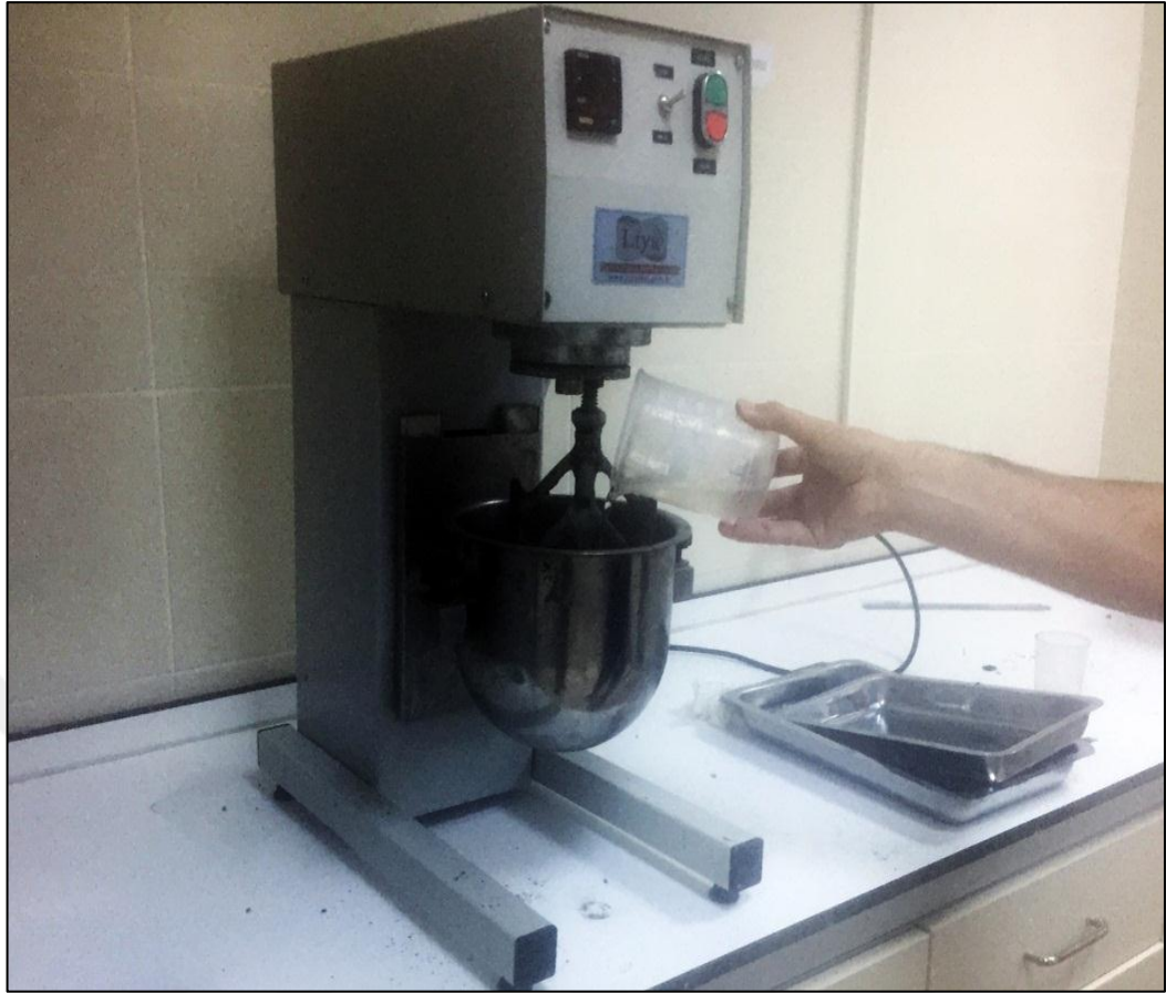
Figure 3.5 Adding alkaline activator to the dry components
