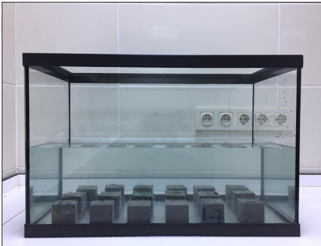
Figure 3.10 Water absorption test by total immersion
