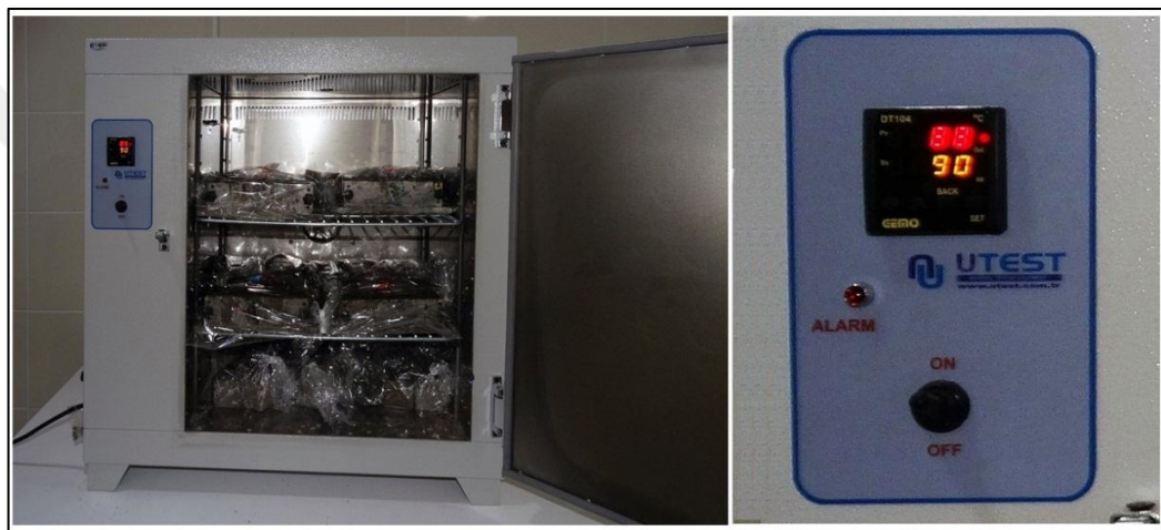
Figure 3.7 Curing cubic specimens by oven dry
