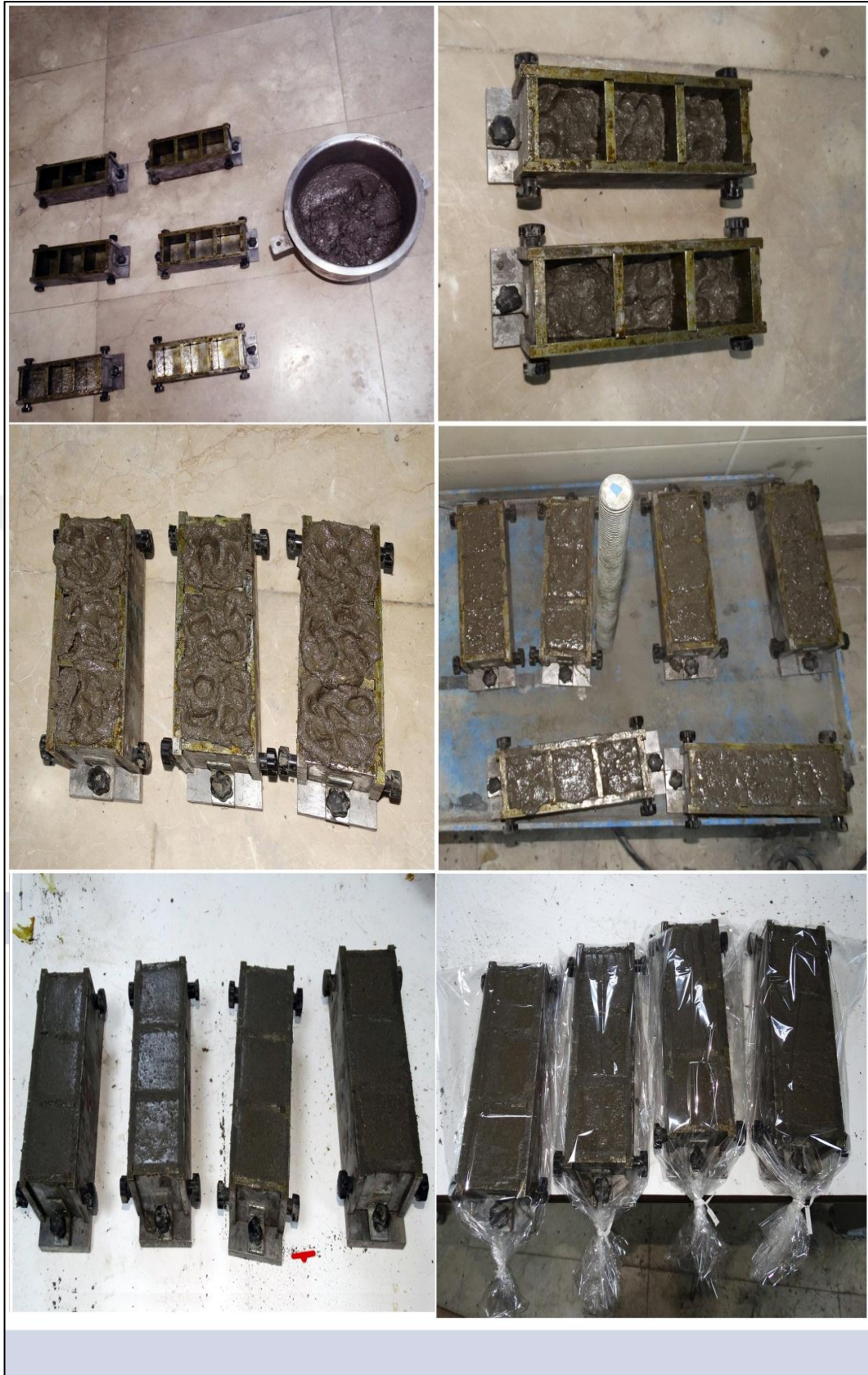
Figure 3.6 Casting geopolymer mortars
