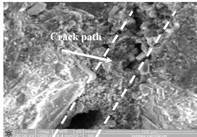
Figure 2.14 ESEM micrograph of rehydration products in a self-healed crack after 30-day sodium hydroxide solution exposure period (Şahmaran and Li, 2008-b)
