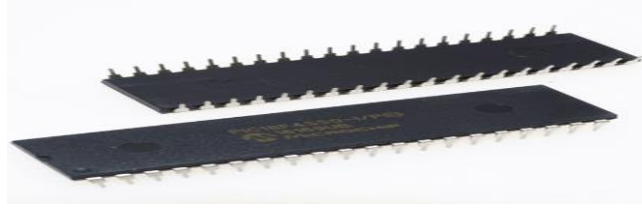
Figure 4.7 PIC18F4550 microcontroller with 40 pins
