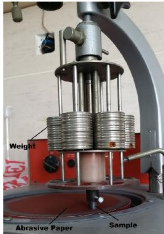
Figure 3.10. Modified grinding and polishing device for abrasion tests
