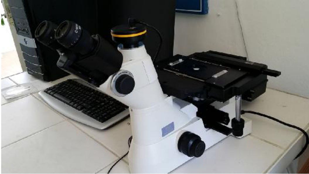
Figure 3.9. Optical Microscope used in the study of microstructure
