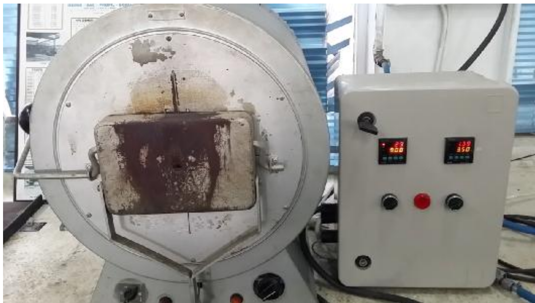
Figure 3.6. Electrical muffle furnace used in the experiments
