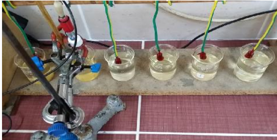
Figure 3.11. Electrochemical corrosion process
