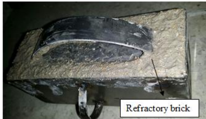
Figure 3.5. Refractory bricks applied around the Seal Container
