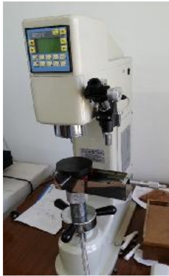
Figure 3.7. Hardness Test Machine used for hardness measurements
