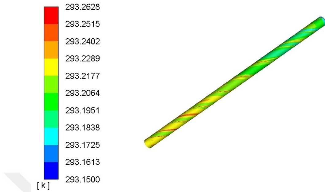
Figure 4.2 Variation of temperature along the pipe
