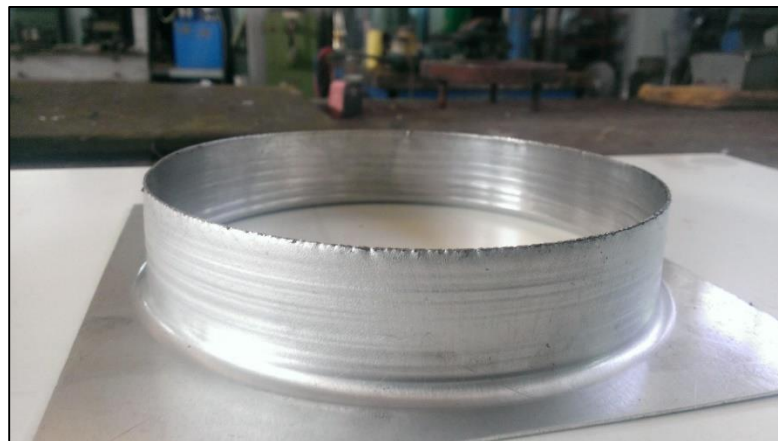
Figure 5.2: 95 mm holed part – No failure occurred.
