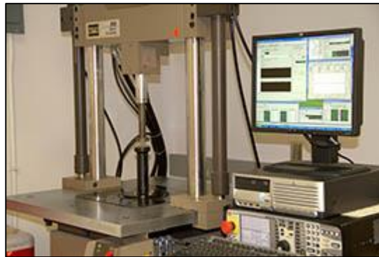
Figure 4.1: Instron machine used for tention test on samples.
