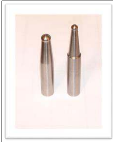
Figure 2.2: Simple forming tools used in SPIF [8]
