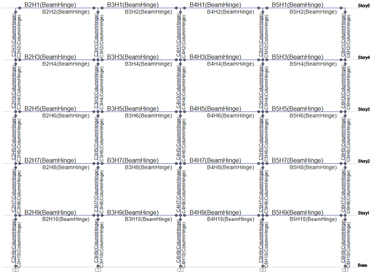
Figure 3.6 Hinge assignment of an elevation
