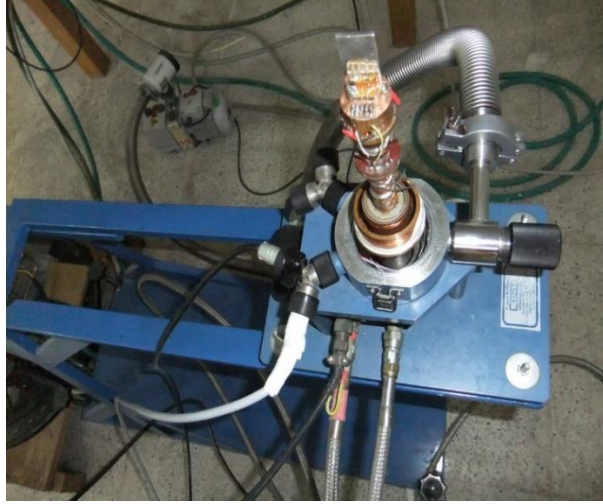
Picture 3.6 Sample mounting on the cold head
