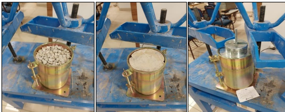
Figure 3.36 Test procedure for testing granular material at the maximum density with the surcharge weight
