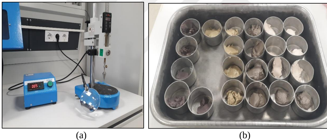
Figure 3.33 (a) Fall cone test equipment. (b) Tested soil
