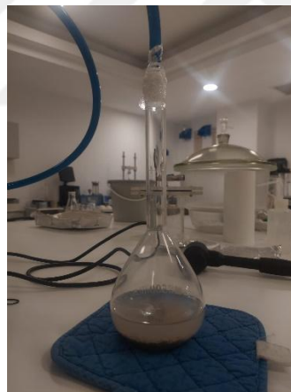
Figure 3.34 Tested material in the pycnometer
