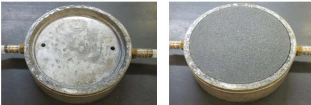
Figure 2.6 Sample base plate without porous stone (left) and with porous stone (right) [4]
