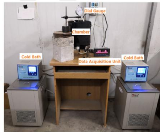
Figure 2.9 Freezing cell scheme [24]
