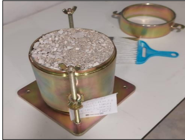
Figure 3.35 Testing granular material at the minimum density
