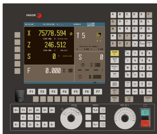
Figure 3.31 Fagor 8055-M display view and control unit specifications
