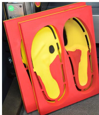
Figure 2.22 Personalized insoles with EVA material
