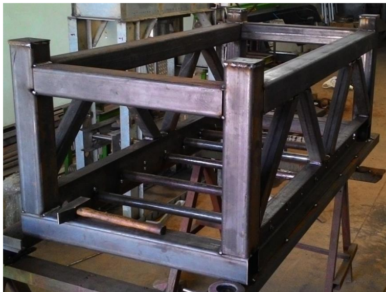
Figure 3.42 Machine frame welding method (Personal archive, 2017)
