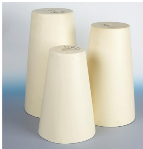
Figure 2.24 Rigid polyurethane foam for prosthetic waist corset
