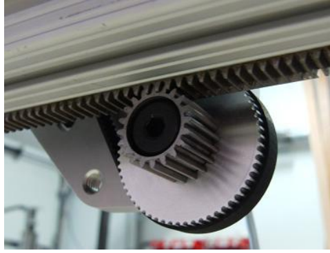
Figure 2.16 Rack & Pinion motion transfer system
