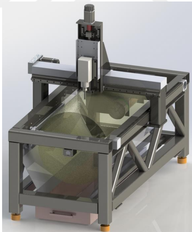
Figure 3.3 New design with 4-Axis (X, Y, Z and A) machining configuration
