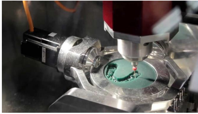
Figure 2.17 Implant teeth manufacturing in CNC Machine
