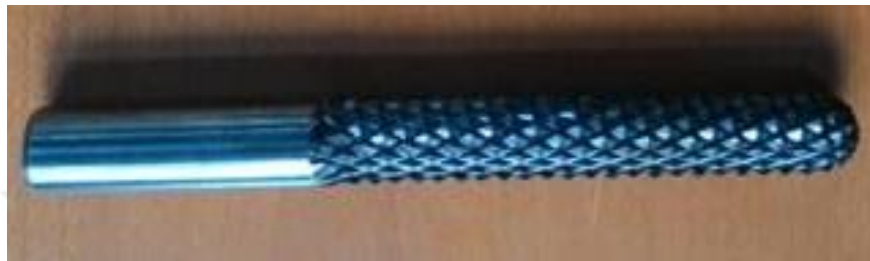
Figure 2.23 Special cutting tool for EVA material
