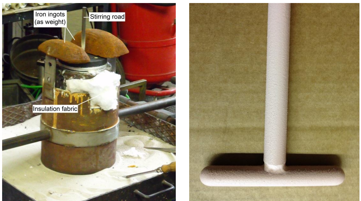
Figure 3.2 The AMS module and coated stirring rod
