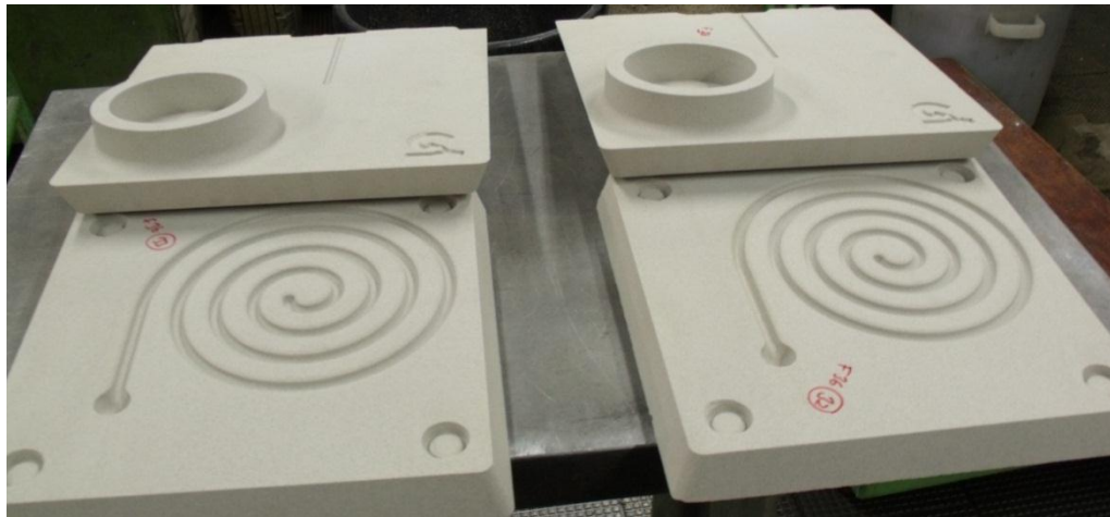
Figure 2.11 Sand spiral mold parts
