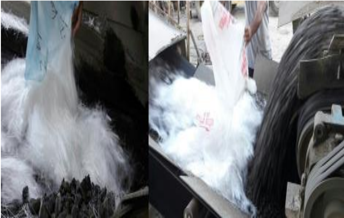
Figure 3. 9: Homogeneously addition of fibers into concrete mixer.
