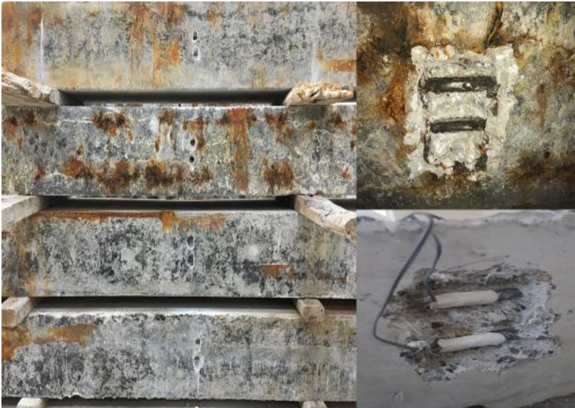
Figure 3. 20: Application of strain gauges.
