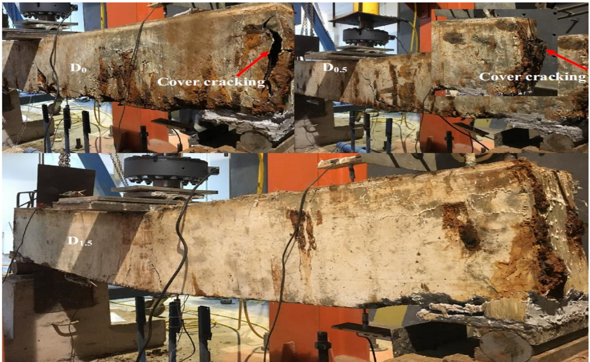
Figure 4.11: Damage levels at failure without releasing jack.
