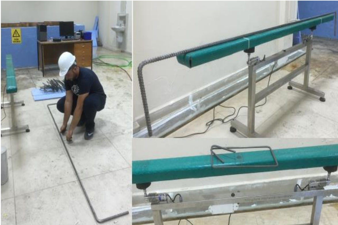
Figure 3. 5: Weighting of reinforcement bars.
