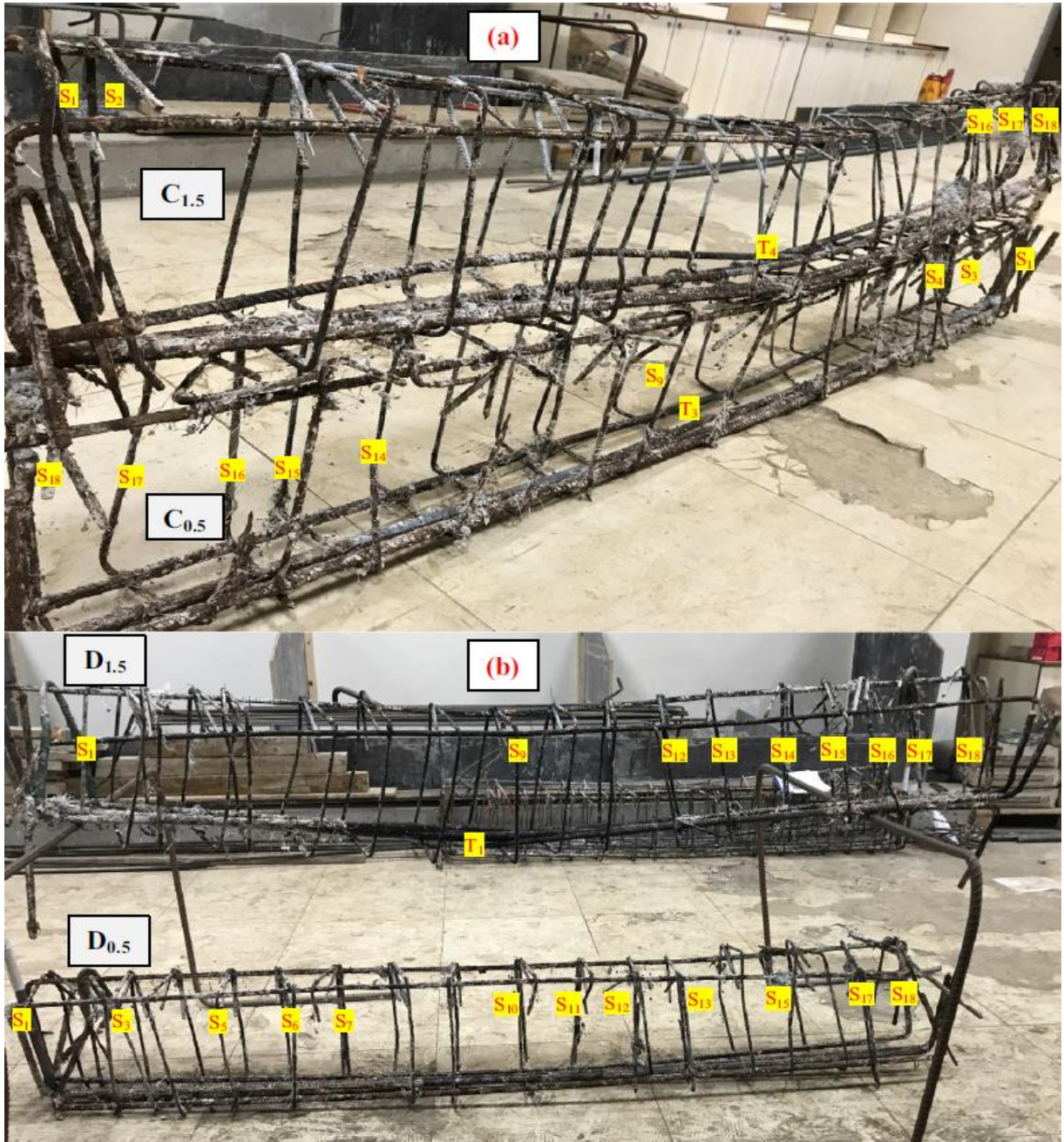
Figure 4. 9: Extracted reinforcement bars: (a) C_{0.5} ( V_f : 0.5%, C_L : 7.4%) and C_{1.5} ( V_f : 1.5%, C_L : 8.4%); (b) D_{0.5} ( V_f : 0.5%, C_L : 9.8%) and D_{1.5} ( V_f : 1.5%, C_L : 10.6%).
