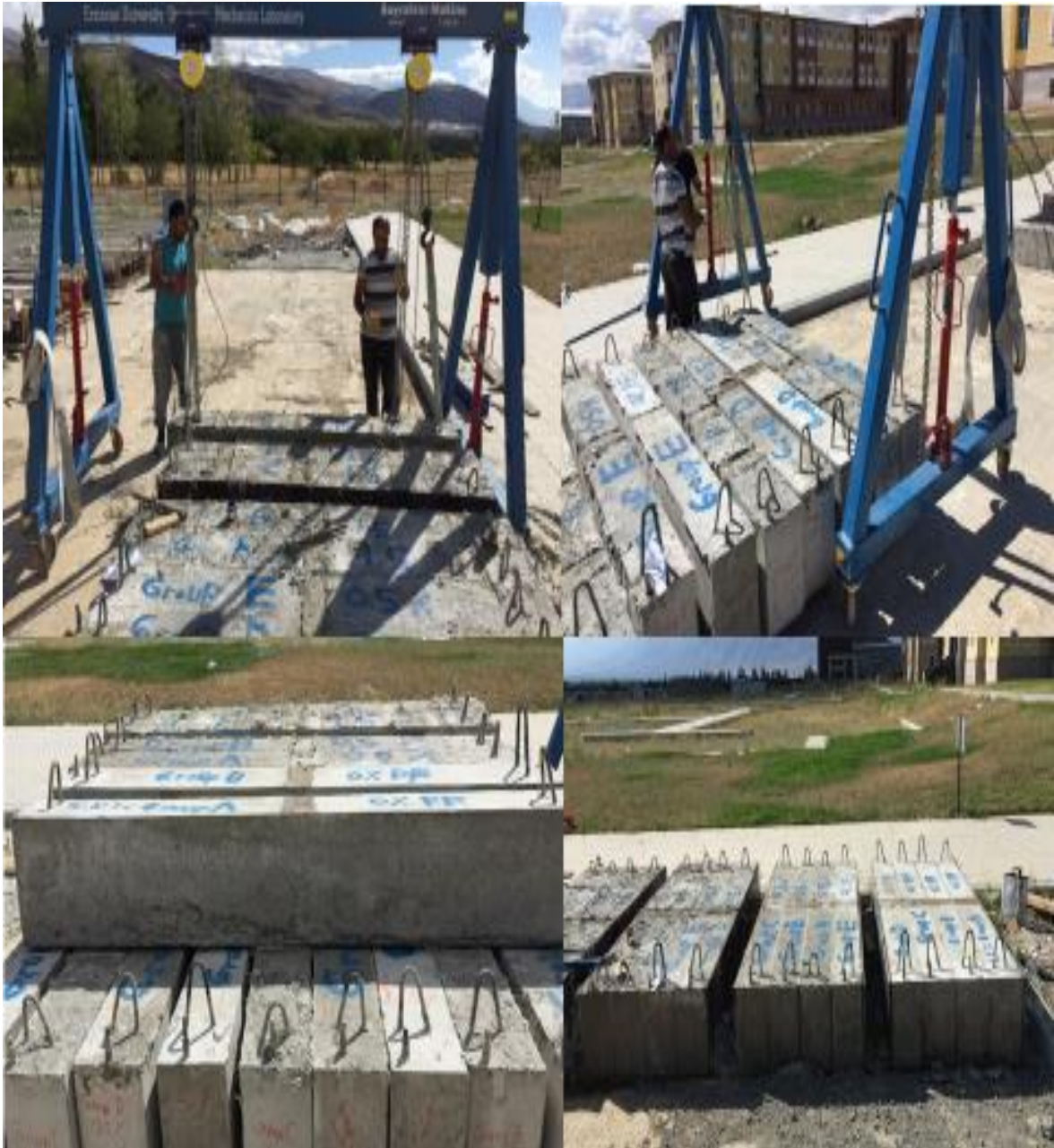
Figure 3. 15: Removal of the RC beams from the moulds.
