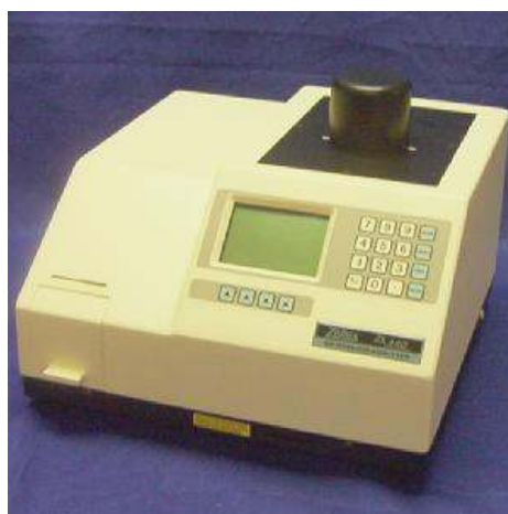
Figure 4.3. Octane Numbers Analyzer
