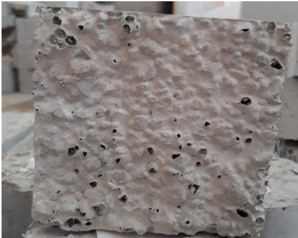
Figure 4.19: PS-SCC Specimen after Heat Exposure at 200 °C
