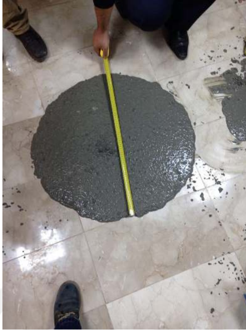
Figure 3.3: Measurement of slump flow diameter
