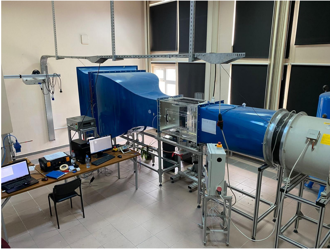
Figure 3.9. General View of Open-Suction Type Wind Tunnel
